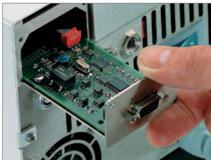
Easy replacement of interface modules
